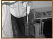
up to 8% fat. A cream test bottle will allow fat readings up to 50%. The smallest division of graduation of a milk test bottle represents .1 of one percent. A cream test bottle is graduated in .5 of one percent.
